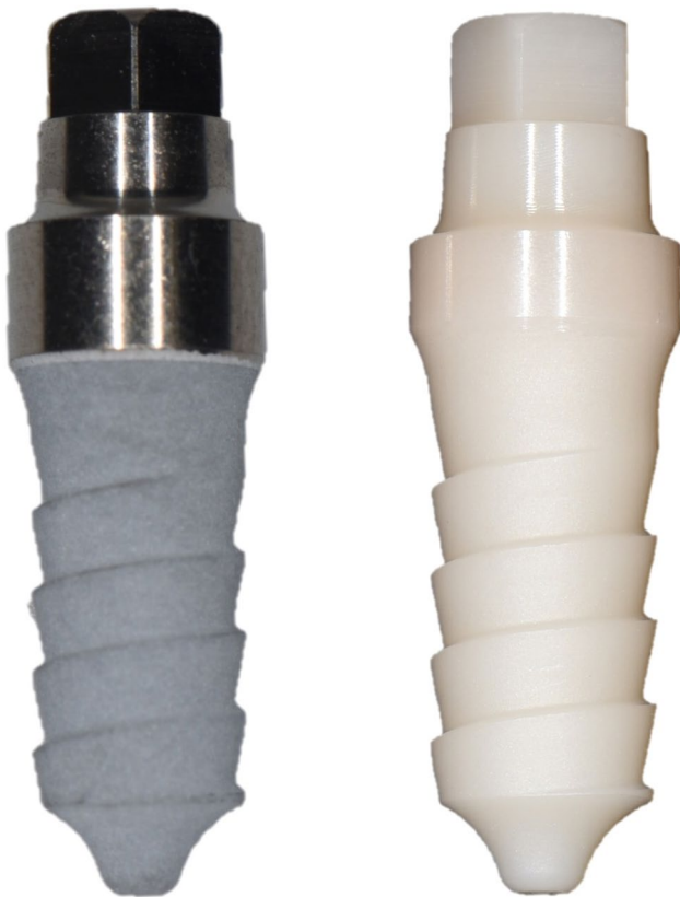
Fig. 2 One-piece yttria-stabilised zirconia implants (Zit-Z, Ziterion GmbH, Uffenheim, Germany) with a 1.5 mm polished collar and a roughened surface (aluminum oxide blasting) and one-piece titanium implants (grade 4) (Zit-T, Ziterion GmbH, Uffenheim, Germany) with a 2.5 mm polished collar and electrochemically coated surface
